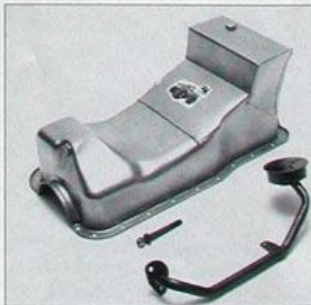
Oil pan conversion is a must for four-wheel-drive V8 swaps in a Bronco II, moving sump away from front end. L&L pan holds 6 quarts, is baffled, has main cap support.
