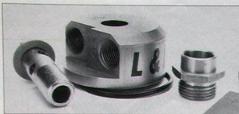
Remote oil filter adapter (1 1/2-inch height) and remote canister mount are musts for engine swaps. The L&L units are machined from aluminum billet; they'll fit Ford and other applications.
