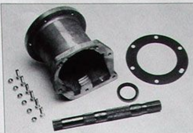
Advance Adapters offers three different C4 adapters, which vary in length from 6 1/4 inches to 11 1/2. This allows your stock Bronco II transfer case to stay in its stock position and retains the stock driveshafts.
