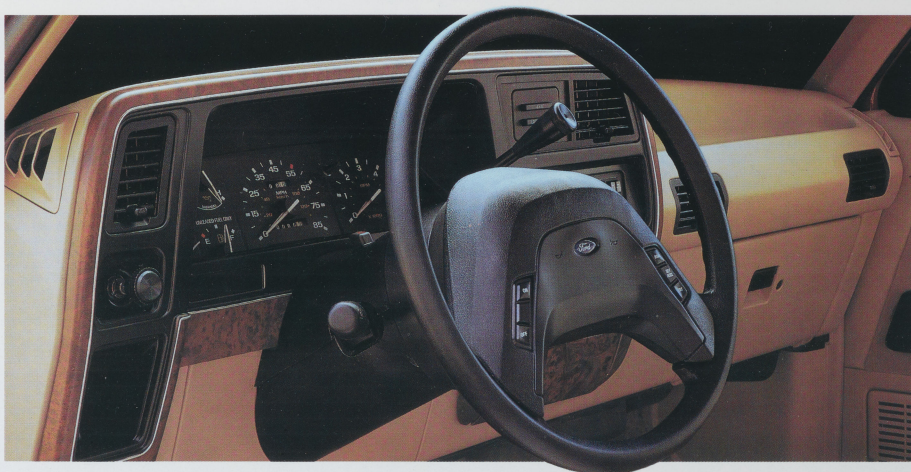
Left: Bronco II for 1989 features a new ergonomic instrument panel designed for excellent driving convenience. The shift lever for the optional automatic transmission is now positioned on the steering column.
