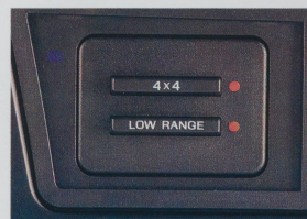
Below: Controls for the optional Touch-Drive electric shift transfer case (4WD) are located on the new ergonomic instrument panel.
